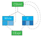
Fig. 4. Fragment of a typical representation of C. The solid arrows represent the instance-of relationship; dotted represent containment.
