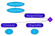
Fig. 3. A term in the incremental parametric syntax for C. The ellipses (light blue) represent language-specific nodes; rhombi (purple) represent generic nodes; rounded rectangles (dark blue) represent sort injection nodes.
